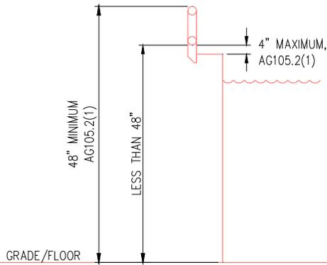
2. Openings in the barrier shall not allow passage of a 4-inch-diameter sphere.
